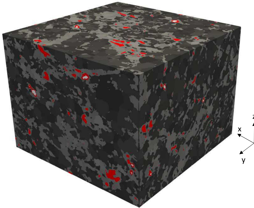
Figure 3: Three-dimensional visualisation of the LTDE-SD1 sample after mineral segmentation. Only the part of the sample considered in the calculations is shown ( 1.7 \cdot 10^{-2} m x 1.7 \cdot 10^{-2} m x 1.3 \cdot 10^{-2} m). Biotite grains are displayed in red.
